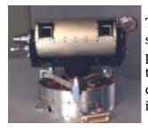
The Imager for Mars Pathfinder or IMP is a stereo imaging system with color capability provided by twenty-four selectable filters for the two camera channels. It is derived from the descent imager/spectral radiometer (DISR) instrument aboard the Cassini Huygens probe.
